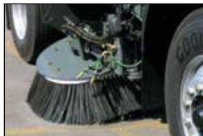
In-cab side broom tilt and extended reach
