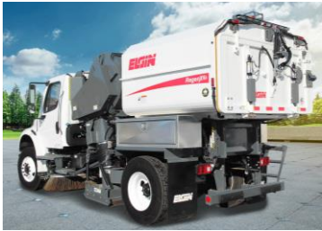
Elgin RegenX1® Regenerative Air Street Sweeper
