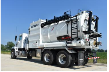
Guzzler Microtrenching Vacuum Truck
