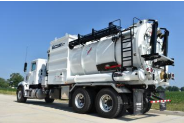
Guzzler Microtrenching Vacuum Truck
