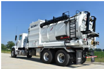
Guzzler Microtrenching Vacuum Truck
