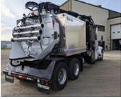
The Westech Coyote's debris body is positioned on the optimal spot of the chassis to ensure the payload is proportionately distributed across all axles simultaneously.
