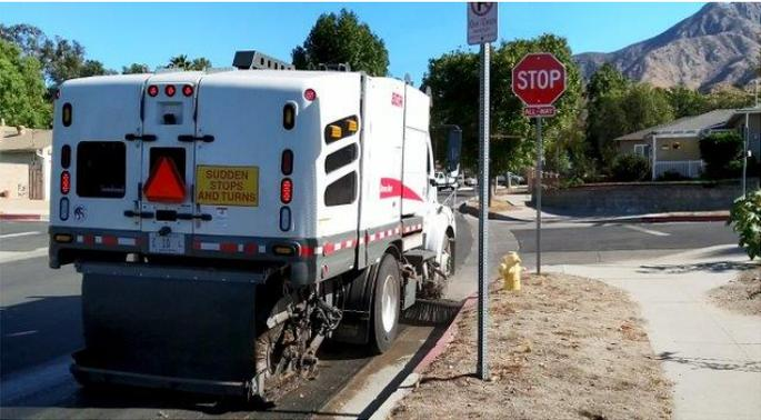
Using a high-capacity battery that can be recharged while driving or when plugged into an electrical outlet, Elgin Sweeper’s hybrid Broom Bear sweeper is designed to tackle everything from heavy-duty construction debris, such as millings or gravel, to light street maintenance.
