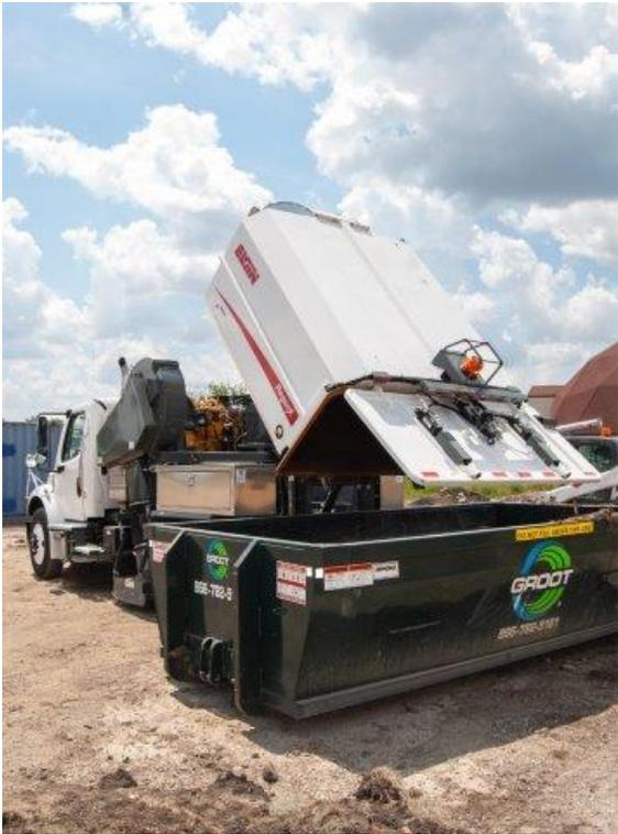
The RegenX is the only sweeper in the industry to offer the ability to dump into roll-off containers while still boasting an impressive 8yd3 capacity.
